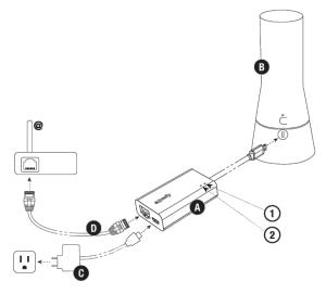
**WIRED CONFIGURATION**using an Ethernet cable
